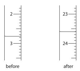
Use the diagram to complete the table. Give the readings to the nearest 0.05 cm<sup>3</sup>.
